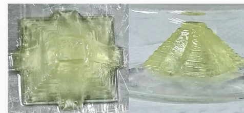
Figure 1: 3D PEG hydrogel printed from precursor solution of JenKem® 8ARM(TP)-ACLT-10K, and M-QTX.
